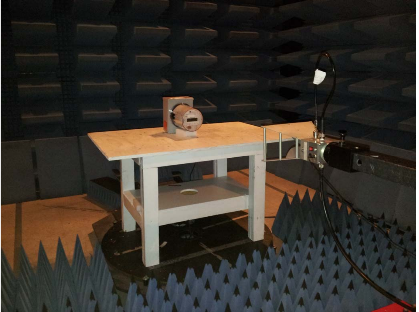
Emissions Test Setup – Intentional/Unintentional Radiated Emissions 1000 - 10000 MHz
