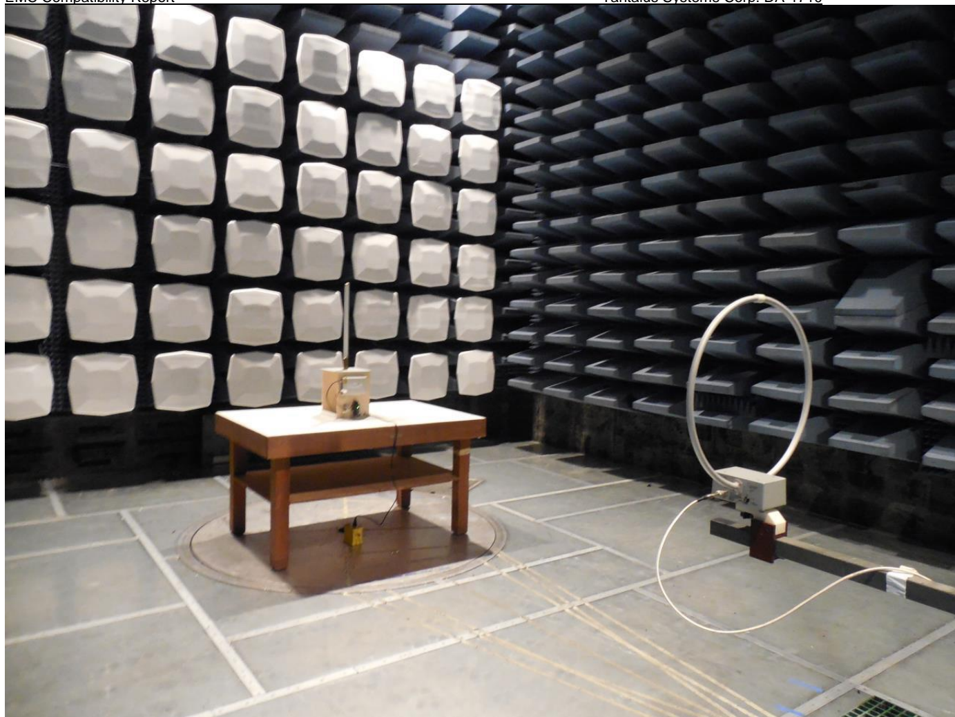
Figure 48: Emissions Test Setup – Intentional / Unintentional Radiated Emissions
