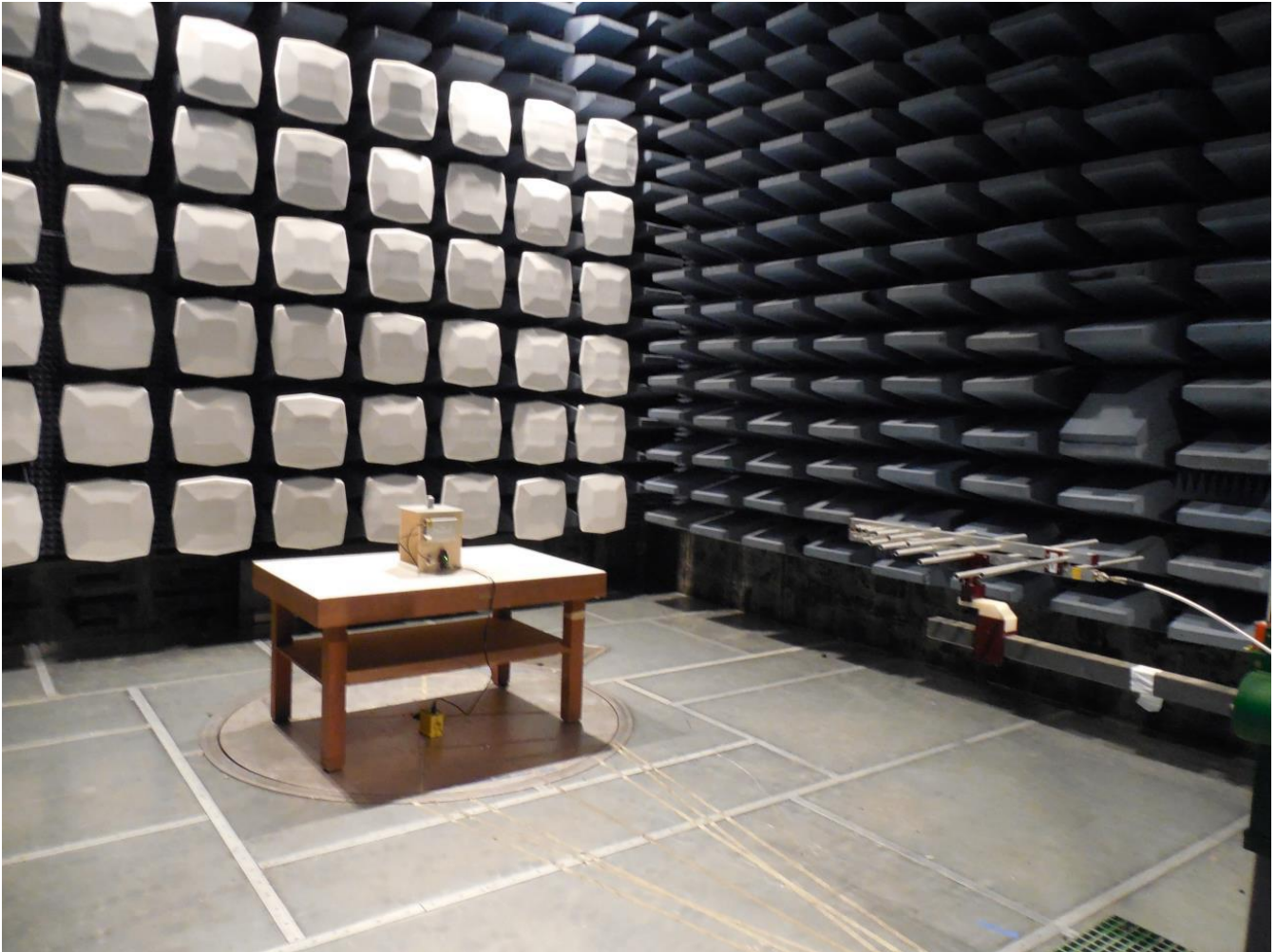
Figure 49: Emissions Test Setup – Intentional / Unintentional Radiated Emissions
