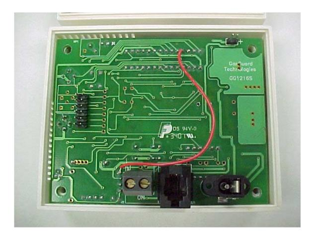
Photo Eight Component Side of RF PCB showing Antenna
