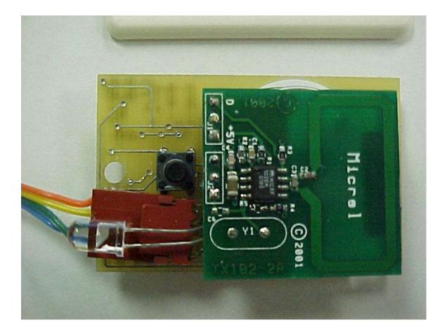
Photo Sixteen RF PCB from Micrel, same PCB as in Gas Detector Battery Contacts as seen from side
