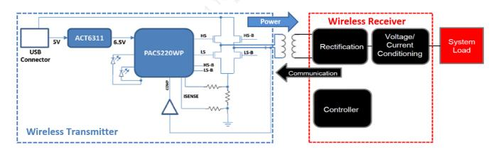
WPC-based wireless power systems consist of a charging pad (primary, transmitter) and the secondary-side equipment (receiver). There are coils placed in the charging pad and secondary equipment, which magnetically couple to each other when the receiver is placed on the transmitter.
