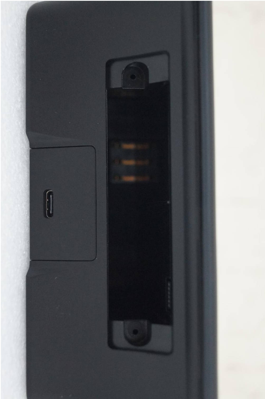
< I/O , Battery slot view >
