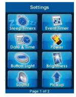
highlight the desired item, then press the **SEL** (Select) button in the center of the navigation pad. To go back a step or to exit the settings screen, press the **Main** button.
