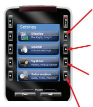
DISPLAY- Press this setting button to adjust the screen and button backlighting. The longer your screen is lit, the more frequently you'll need to charge the MX-980.
