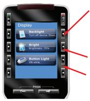
BACKLIGHT - Specify how long the MX-980 screen should stay lit after you press a button. You can select two different time out settings. One for when it is hand held, another for when it is in the charging base.
