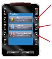
POWER- Displays the current power remaining and enables you to set the level that triggers a warning when you are using the MX-980.
