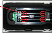
Place the four AAA batteries into their positions in the battery compartment observing the + and polarity indicators on the batteries.
