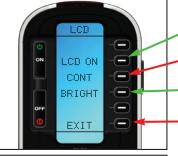
To activate the LCD On/Off setting, press this button. See below.
