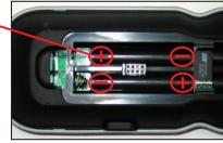
Place the four AAA batteries into their positions in the battery compartment observing the + and polarity indicators on the batteries.
