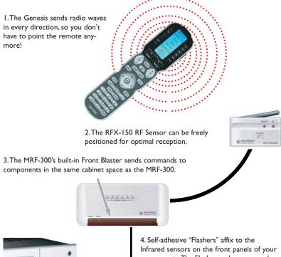
Infrared sensors on the front panels of your components. The Flashers relay commands to components out of sight of the MRF-300's Front Blaster. The flashers plug in to the MRF-300's rear flasher line outputs via their 10 foot cables. Uniquely, the MRF-300 can also connect to rear panel IR Inputs via its adjustable IR Line Outputs.
