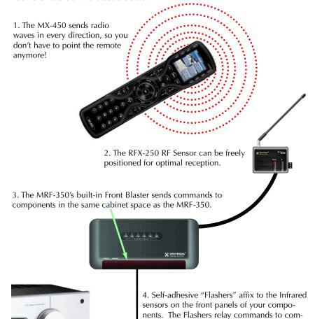
ponents out of sight of the MRF-350's Front Blaster. The flashers plug in to the MRF-350's rear flasher line outputs via their 10 foot cables. Uniquely, the MRF-350 can also connect to components with rear panel IR Inputs
