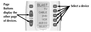
Select the new setting by pressing the desired button, then press SAVE to save your new setting and return to the RF settings menu.
