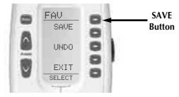
To save the channel you entered, press the SAVE button. The UNDO button lets you erase the last entry. The EXIT button erases all entries for this button.
