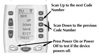
When the component turns off, save the code number you entered by pressing the SAVE button that appears on the screen.
