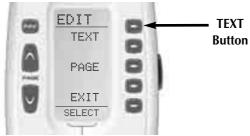
The screen displays the list of devices and "EDIT" will appear at the top of the screen. Navigate to the device and page where there is a button label you want to EDIT, selecting between the FAV, MAIN, DEVICE, then using the PAGE button.
