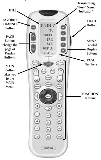
\*Note: When a command, macro or favorite channel is being transmitted, an icon will appear in the top right corner of the display. While the Osiris is "busy", it will ignore a button push.
