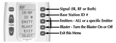
After you've made a new setting and SAVED your change, use the EXIT button to return to the RF settings menu to change any other setting. Once you are finished all settings, use the MAIN button to return to normal operation
