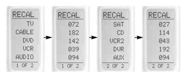
**Note:** Pay attention to the page numbers on the bottom of the screen. Page 1 code numbers are the ones setup for the Page 1 Devices. Page 2 code numbers are the ones setup for the Page 2 Devices.
