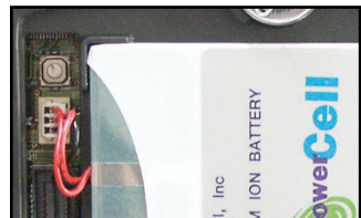
Battery Cable Plugged In
