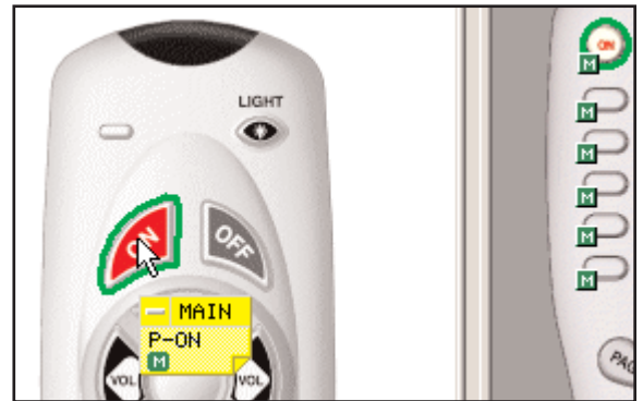
In this illustration, you can see that the MACRO from MAIN power on has been successfully dropped into the SideKicks ON button.
