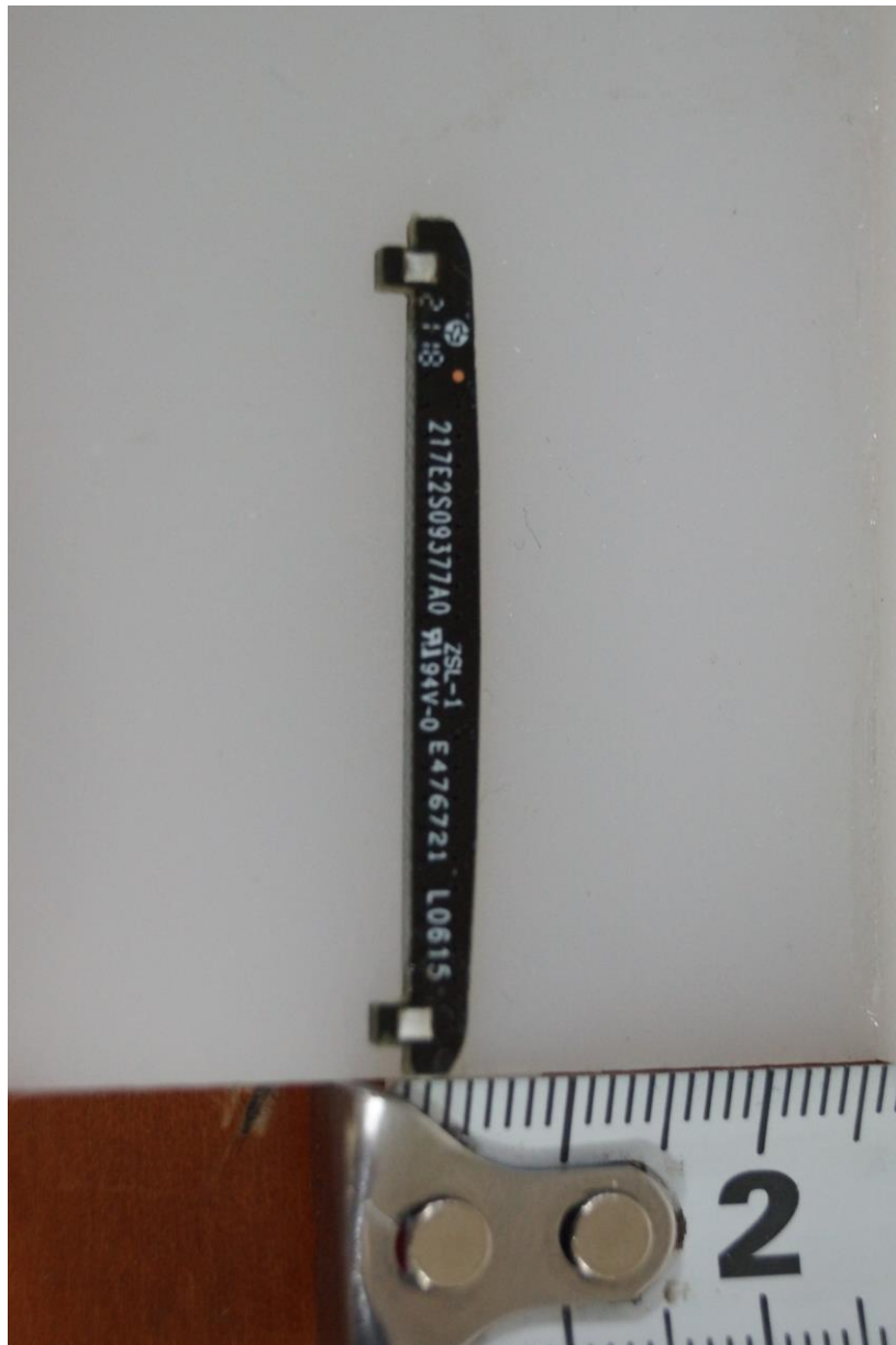
< RF 433 antenna bottom view >
