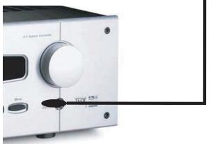
4. Self-adhesive "Flashers" affix to the Infrared sensors on the front panels of your components. The Flashers relay commands to components out of sight of the MRF-300's Front Blaster. The flashers plug in to the MRF-300's rear flasher line outputs via their 10 foot cables. Uniquely, the MRF-300 can also connect to rear panel IR Inputs via its adjustable IR Line Outputs.
