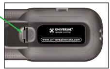
Note that the three contacts on the battery must connect to the three spring-loaded contacts in the MX-880i. Angle the battery into the battery compartment, contacts first, then gently fit the rear of the battery into the compartment as well. Replace the battery cover by inserting the hinged end in first, then snapping the cover back into place.
