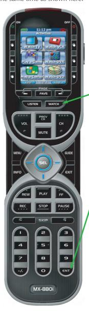
At the same time, press and hold both the WATCH button and the ENTER button. When the SETUP screen appears, you can release the two buttons.
