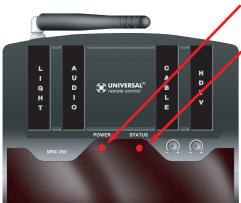
The red POWER LED indicates that the MRZ-260 is powered on.
