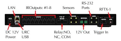
DC 12V Power: Attach the included 12V DC 3.5A power supply here.
