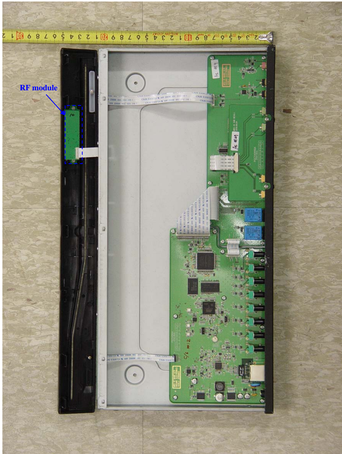
< Inside #3 RF module location >
