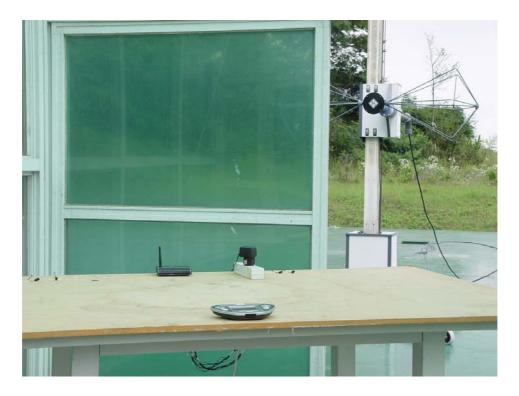
■ Radiated Test Picture (Rear)
