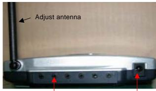
Connect IR Extender cable jack. Connect DC9V Power supply.
