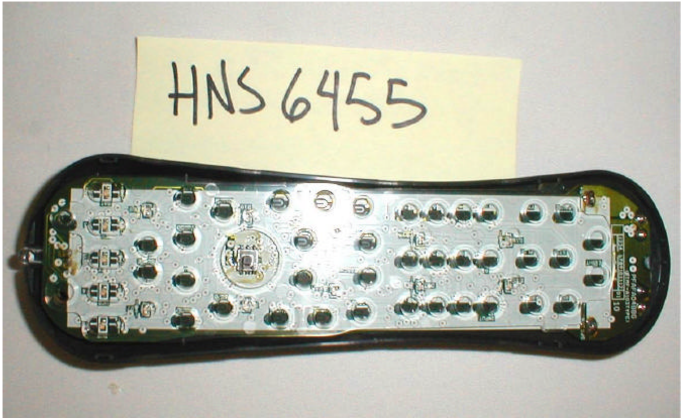
Key Pad Membrane Removed, Top View of PCB
