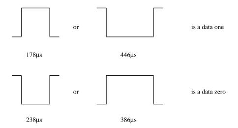
Bits in the data stream always alternate between the high and low state representations. The specific binary data being transmitted determines which of the pulse widths represent a one or a zero.
