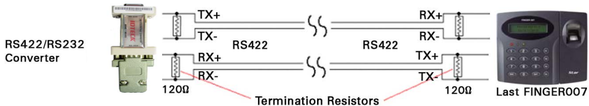
Figure: Termination Resistors for 4 Wire RS422 Communication System
