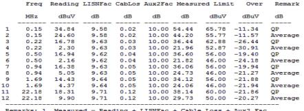
Remarks: 1. Measured = Reading + LISNFac + Cable Loss + Aux2 Fac. 2. The emission levels that are 20dB below the official limit are not reported.
