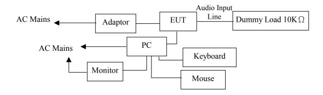
(EUT: 900MHz Transmitter and Receive (Speaker with USB))
