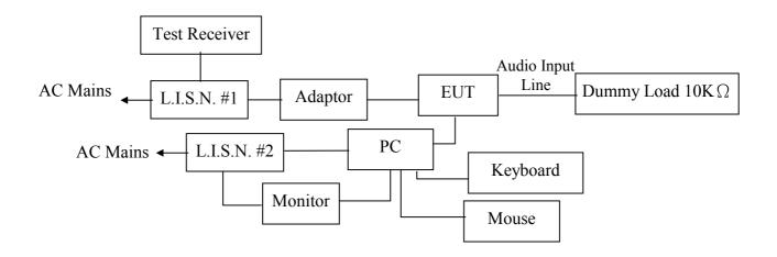
(EUT: 900MHz Transmitter and Receive (Speaker with USB))
