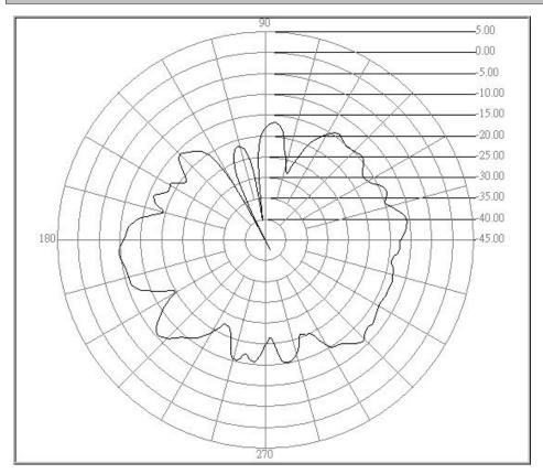
Center freq.(MHz): 2480 Polarization : E Plane
