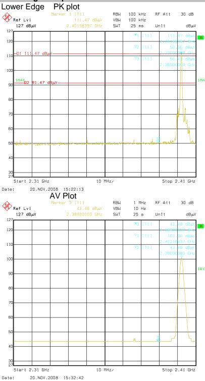
Max carrier field strength PK 95.6dBuV/m, AV 95.4dBuV/m At 2.390GHz, the deviation of PK plot is 60.91dB, AV plot is 57.52dB The field strength at 2.390GHz PK 34.69dBuV/m, AV 37.88dBuV/m Which fulfills the requirement of PK 74dBuV/m and AV 54dBuV/m
