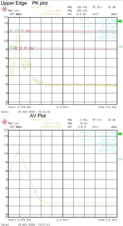
Max carrier field strength PK 83.6dBuV/m, AV 83.4dBuV/m At 2.4835GHz, the deviation of PK plot is 57.78dB, AV plot is 45.6dB The field strength at 2.4835GHz PK 25.82dBuV/m, AV 37.8dBuV/m Which fulfills the requirement of PK 74dBuV/m and AV 54dBuV/m
