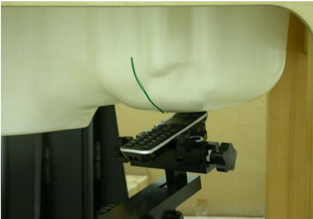
Measurement Position of Left-Tilt (LT) with Handset
