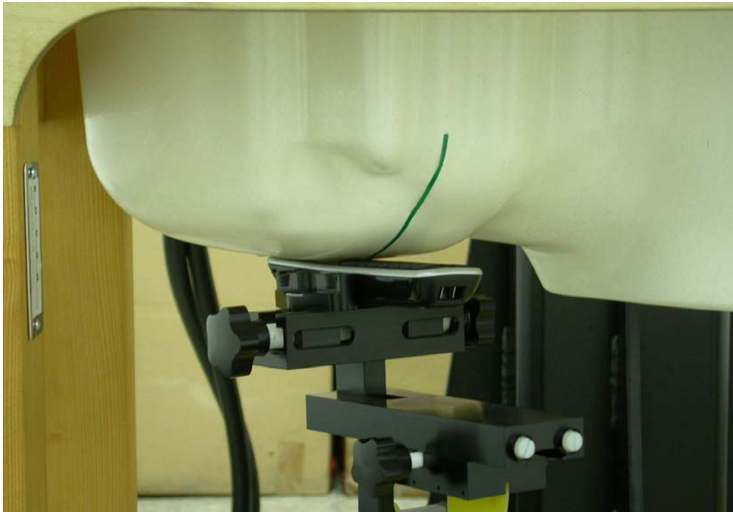
Measurement Position of Right-Cheek (RC) with Handset
