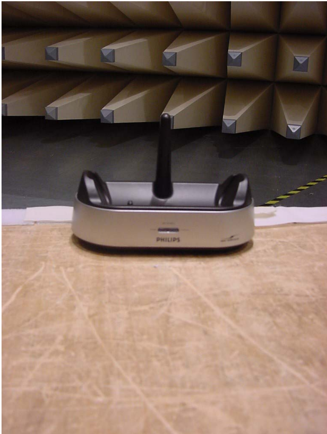
Photo 2 (Radiated Emissions): Tx Test set-up
