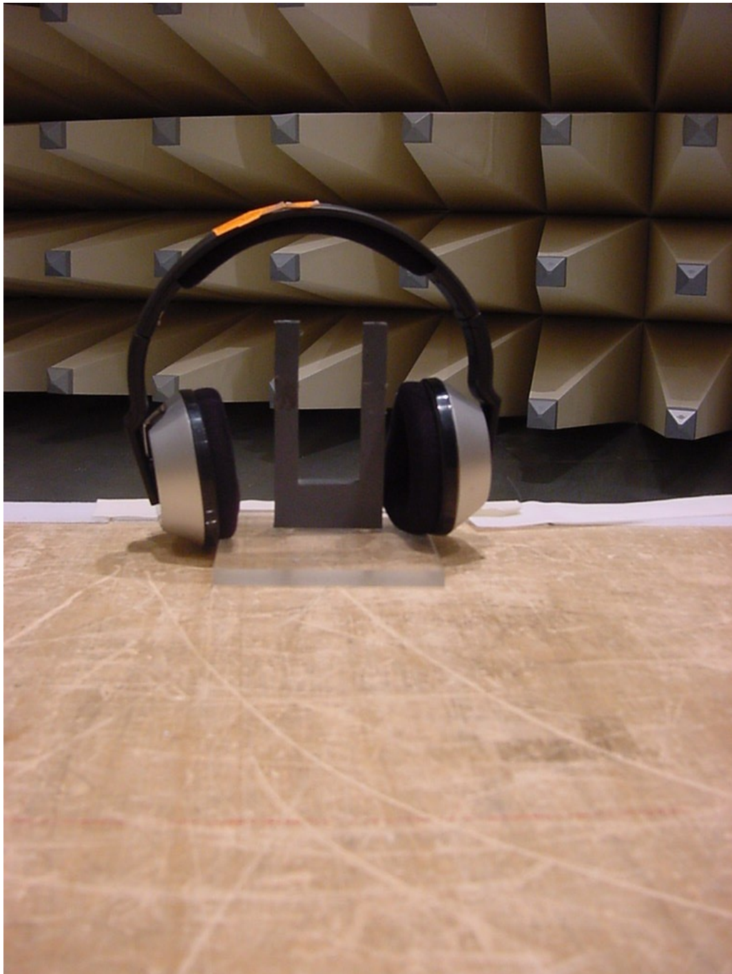
Photo 4 (Radiated Emissions): Rx Test set-up
