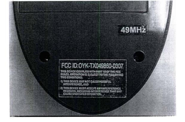
FCC Label size: 30 x 17mm 49MHz label size: 13 x 4 mm
