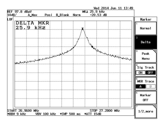
From above plot, at the bandedge 26.96 and 27.28MHz, are more than 20dB down from the 27.145MHz carrier. That mean the Operation frequency is within the band: 26.96 - 27.28 MHz.
