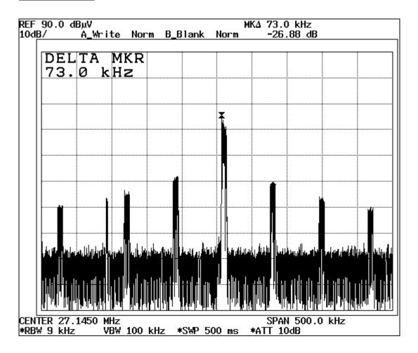
The field strength of any emission within the operation band did not exceed 80 dB(μV/m) for average value or 100 dB( $\mu$ V/m) for peak value.
