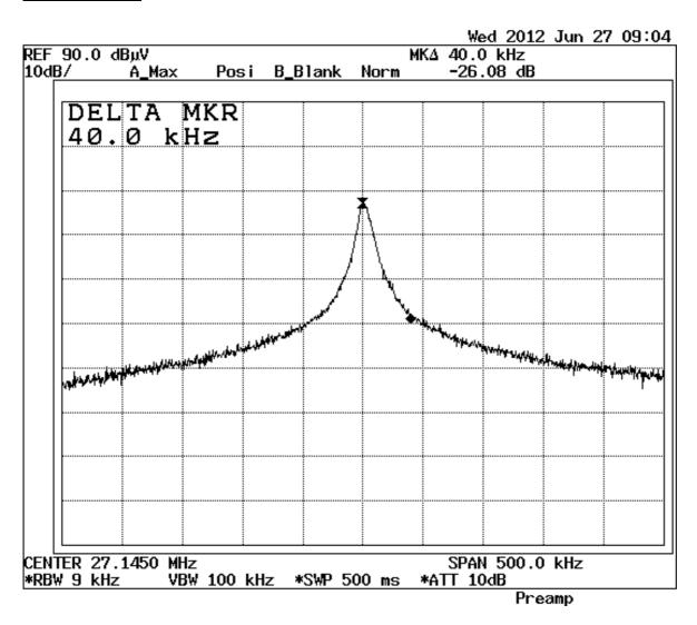
The field strength of any emission within the operation band did not exceed 80 dB( $\mu$ V/m) for average value or 100 dB( $\mu$ V/m) for peak value.
