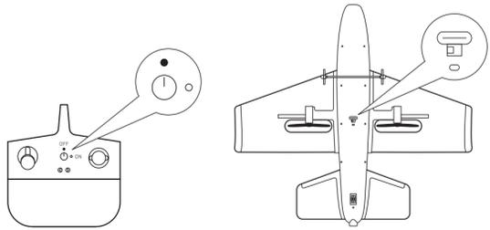
1. Before starting, make sure that the power switches for both the remote controller and plane are in the off position by rotating the power switch counterclockwise.
