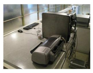
Measurement of Radiated Emission Test Set Up
