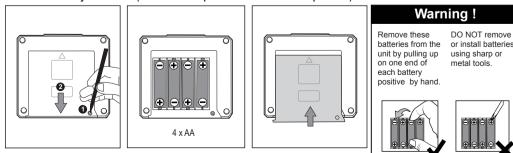
Note: When the power indicator on the transmitter starts blinking, replace the batteries. Plane battery charging
