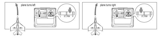
4. Push the direction stick toward left to turn the plane anticlockwise, and push the direction stick toward right to turn it clockwise. The plane turns depending on the speed difference between the left propellers and the right propellers
