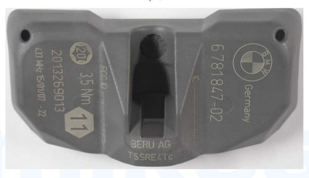
Wheel Electronic / TSSRE4Tc External Photo Rear view
