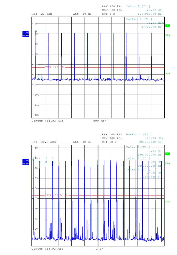
=> 120 transmissions at intervals about 500ms (alarm mode) => Fallback to normal mode after 60s
