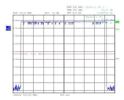
Worst Tx on time – alarm mode: Within 100ms 1 transmission a 5.5ms => Max Tx on time 5.5ms
