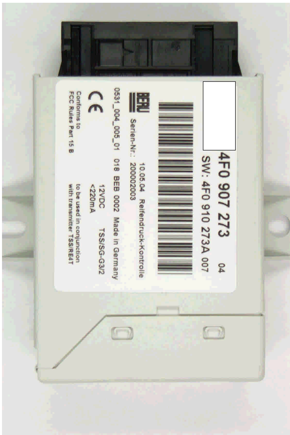
40458eut31.jpg: EUT, TSS/SG-G3/2 front view
