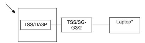
\* Laptop with Vector Tool "CANoe" to establish CAN communication to Control Unit (TSS/SG-G3/2).
