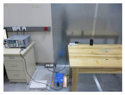
FCC RADIATED EMISSION TEST SETUP
