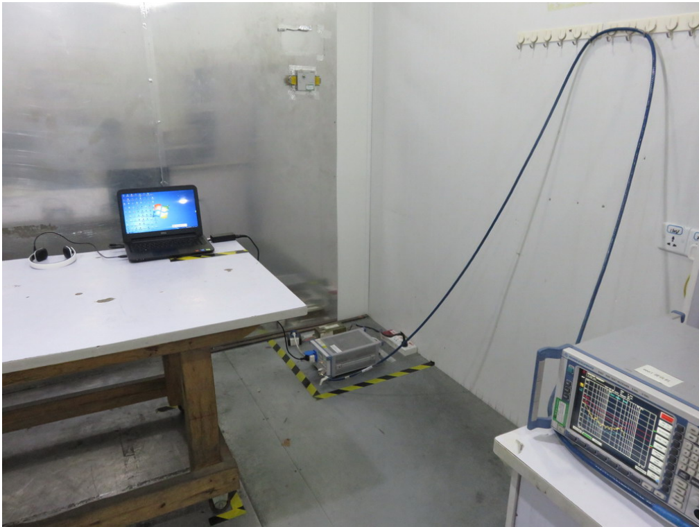
FCC RADIATED EMISSION TEST SETUP
