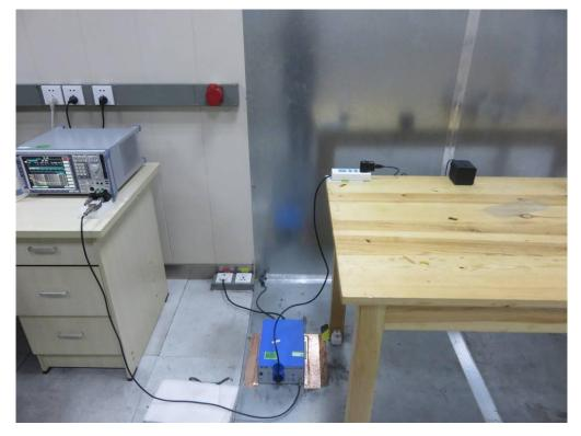
FCC RADIATED EMISSION TEST SETUP
