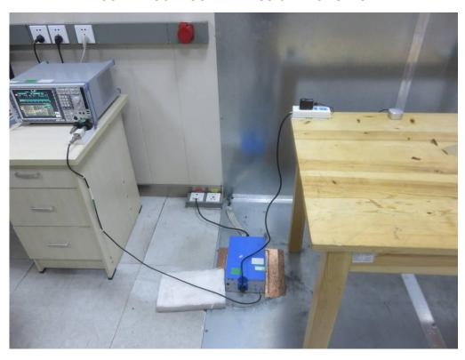
FCC RADIATED EMISSION TEST SETUP
