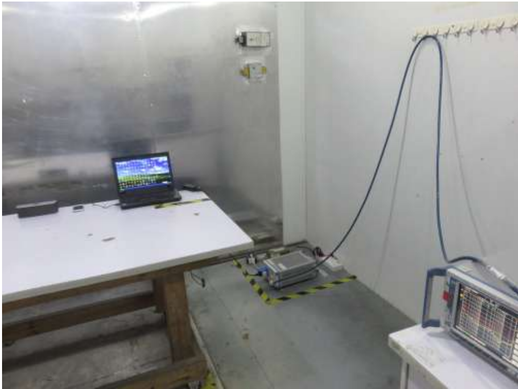
FCC RADIATED EMISSION TEST SETUP
