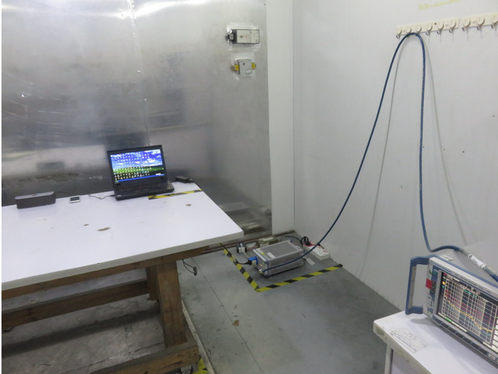
FCC RADIATED EMISSION TEST SETUP
