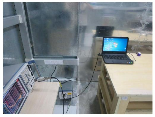
FCC RADIATED EMISSION TEST SETUP
