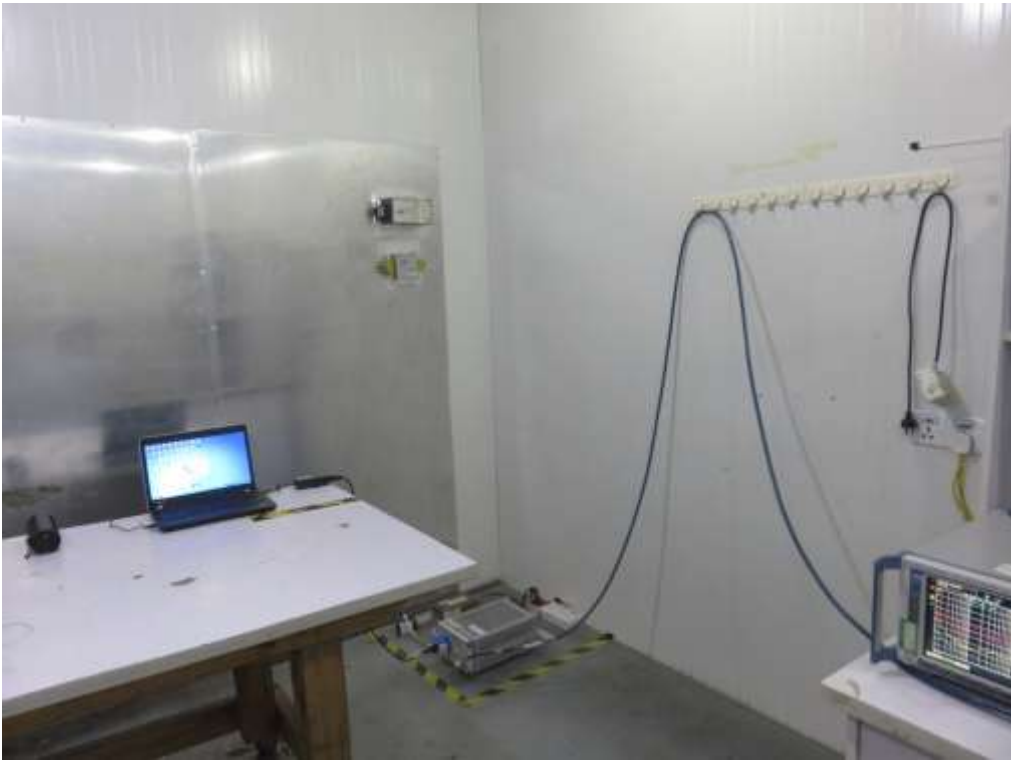
FCC RADIATED EMISSION TEST SETUP
