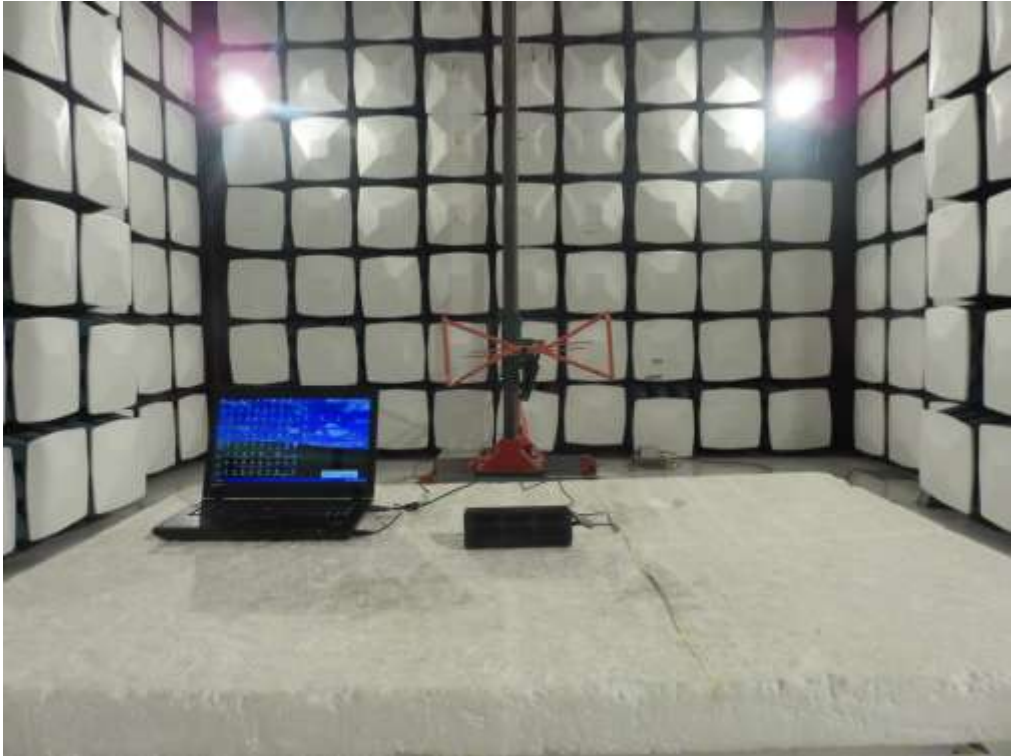
FCC RADIATED EMISSION TEST SETUP
